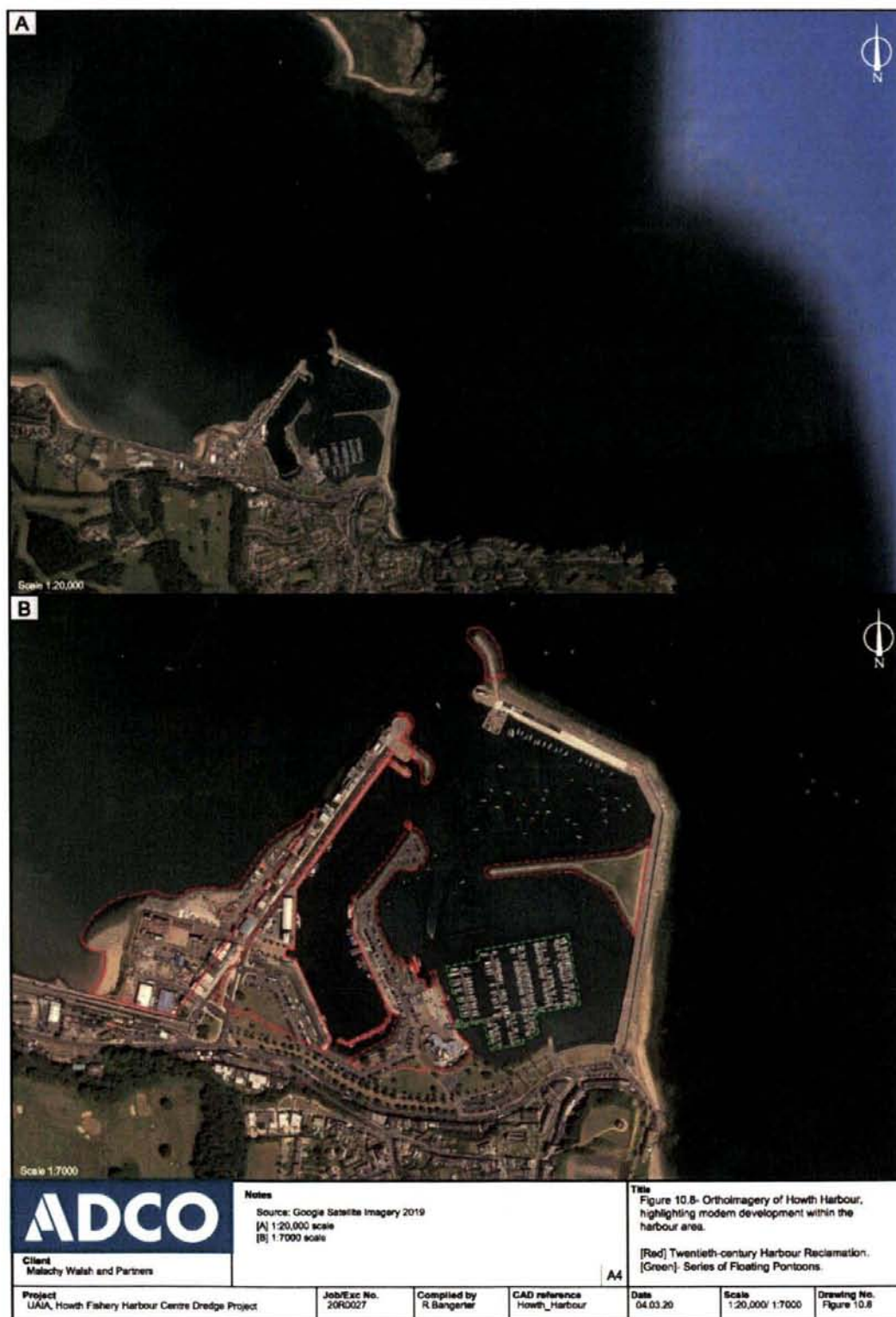
Figure 8: Orthoimagery of Howth Harbour with twentieth-century reclamation works highlighted.
